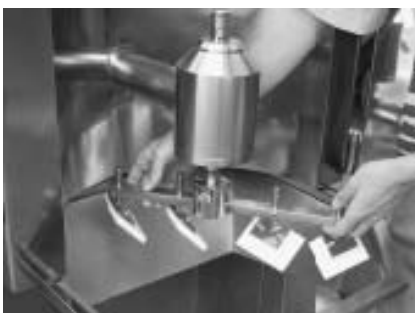
Fig. 11 The stripping device/rake with four wipers must be mounted on the drive shaft from below.
