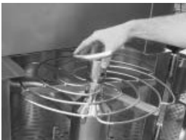
Fig. 14 The rough-crush/pre-break spiral is mounted and saved with the hexagon bolt.
