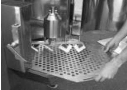
Fig. 12 The perforated plate/screen must be inserted.
