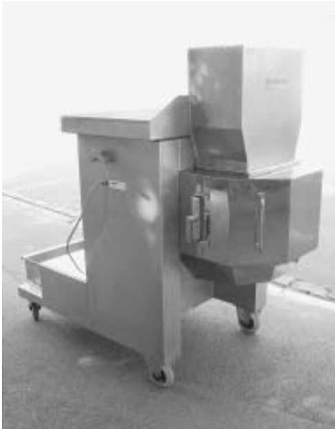
Fig. 2 + 3 = Standard Spiral-Separating-Machine with or without working platform but on wheels.
