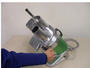
The closing lever simultaneously is the "Emergency-Off" switch. It is located directly adjacent the outlet on the right-hand side of the machine.
