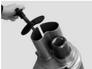
The pusher plate is lifted and swivelled away, so that vegetables can be filled in.
