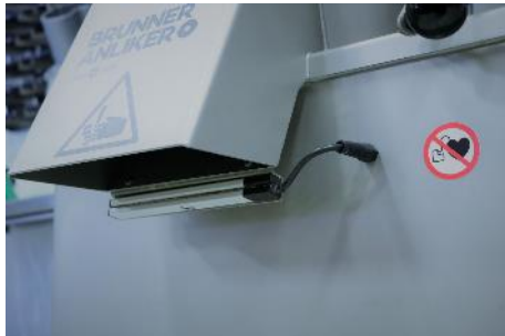
Fig. 4: Antistatic system at the outlet
