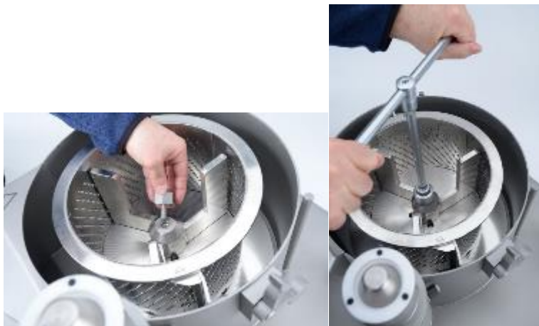
Fig. 24: Fasten the grating blades
