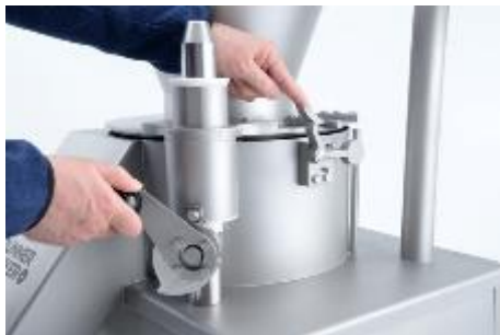
Fig. 17: Open the lock on the funnel
