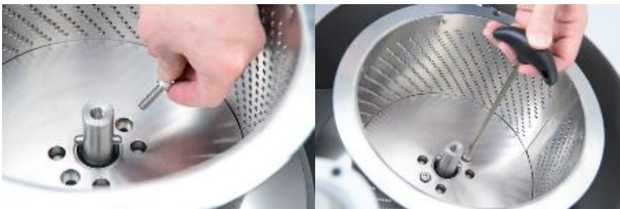
Fig. 22: Fasten the grating drum
