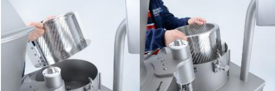
Fig. 21: Insert the grating drum
