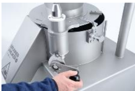
Fig. 18: Lift the funnel by turning the lever clockwise
