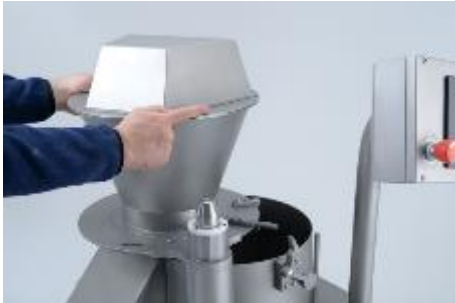
Fig. 19: Swing out the funnel
