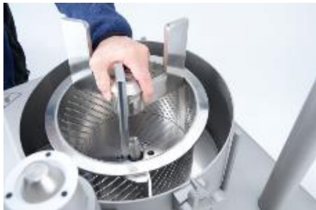
Fig. 23: Insert the grating blades
