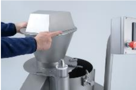
Fig. 25: Swing the funnel over the grating compartment
