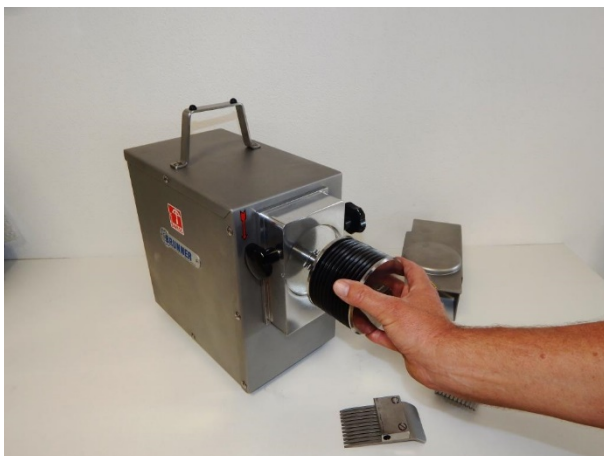
Figure 7 and 8: Holding the rotary cutter
