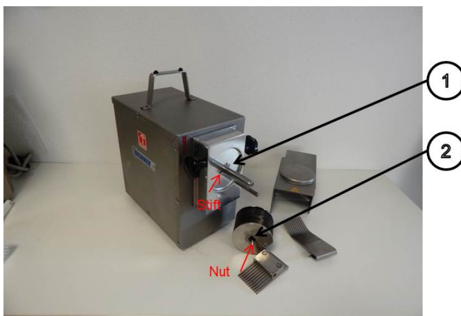
Figure 10: Installation of rotary cutters
