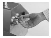
The bearing yokes should first be turned 90 degrees left or right and can then be removed.
