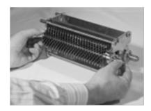
When removing or replacing the knife rolls, grasp them only by the shaft ends.
