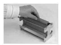
The two rakes should be hung with the curves towards each other and with the cam at the top of the grooves of the roll carrier.
