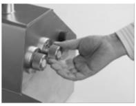
The bearing yokes should be attached without lubrication and secured with a 90 degree turn.
