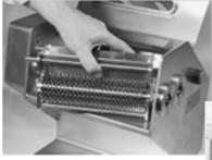
Starting with the right side, mount the complete roll carrier
